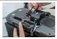
Install the red and blue flashing lights in the M300 tripod and connect the light cable with the control box, the installation position and direction as shown:
